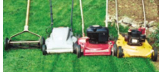
Electric and gas "mulching" mowers (center) chop clippings and blow them down to soil to decompose.
